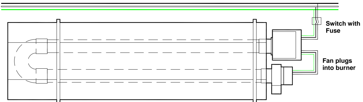
Figure 5.a Typical U-Tube Range Wiring Connections
